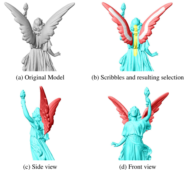
Figure 1: User session with the Lucy point set model. To select the wings of the model (a), the user draws a white scribble to select each wing and a yellow scribble to exclude the body (b). Even though the user marked from only one view, the wings are completely selected (c,d). The entire interactive process for this initial partitioning takes less than 15 seconds even when using this 14 million point model.
